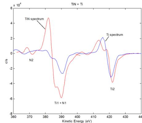
Figure 4 Overlapped spectra of TiN and Ti reference
