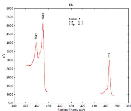
Figure 7. Ti2p3 and N1s spectrum in TiN coating by XPS
