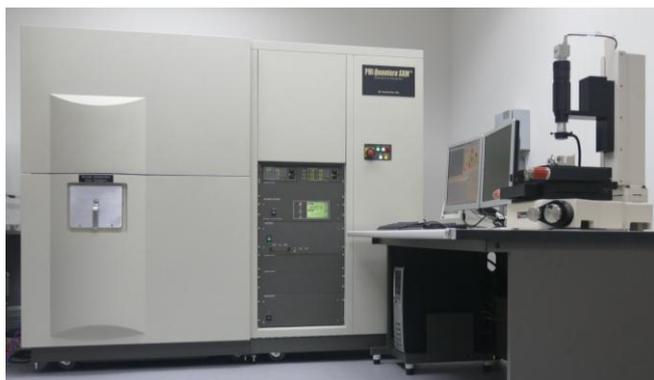
Fig 5. PHI Quantera Scanning X-ray Microprobe
