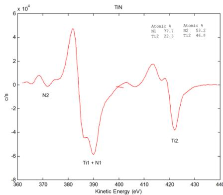
Figure 3 Derivative spectrum of Ti and N in TiN coating
