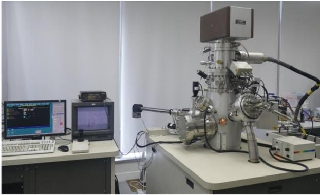
Figure 1. PHI 680 Scanning Auger Nanoprobe
