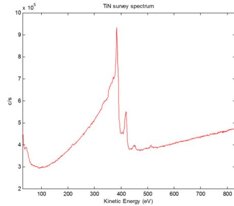
Figure 2. Survey spectrum of TiN coating by AES
